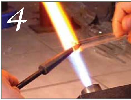
4 Flare open one end of a 12.7mm tube.
