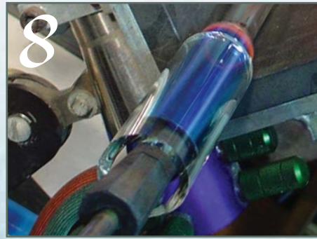
8 Slide clear sleeve into place over whole dichrosilicate tube once 12.7 blowtube has been welded on.
