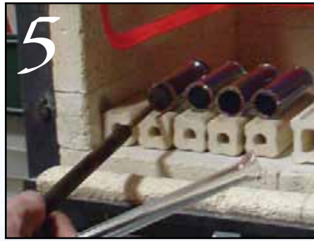
5 Open kiln, take a large reamer and slip the the larger reamer into the dichrosilicate tube, pull it out of the kiln.
