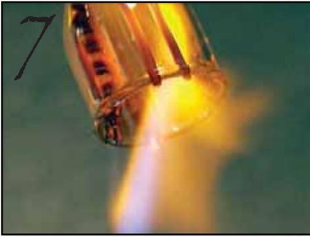
Pick up your silvering rod and using a neutral to slightly oxidizing flame, fume the inside of the point.
