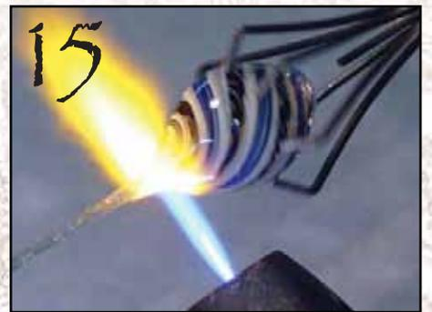
With pre-heated claw- grabbers secure the bead and pull off the remaining handle. Clean off any excess glass. Open the hole as in previous step.
