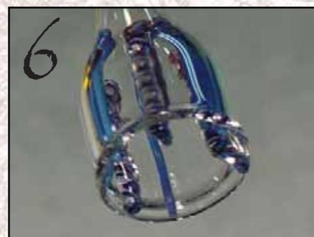
6 Draw in lines of color with stringers, applying them in the spaces between the lines of latticino. Heat and condense slightly to melt in decoration.
