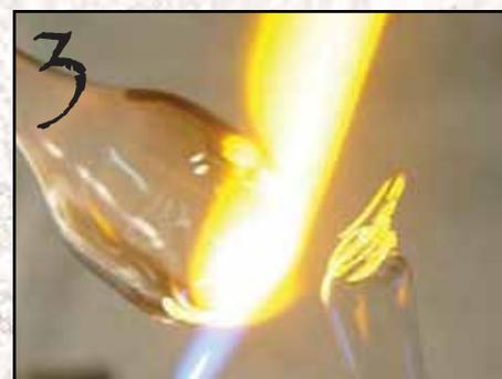
3 Using a rod or scrap, clean off any excess glass from the lip area.
