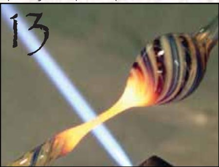
Using a pinpoint flame, remove one of the handles. Use a rod to "pick off" any excess glass.
