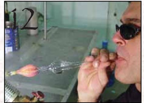
Heat and blow to desired shape. Repeat the process to work the design in and to apply any pattern twist.
