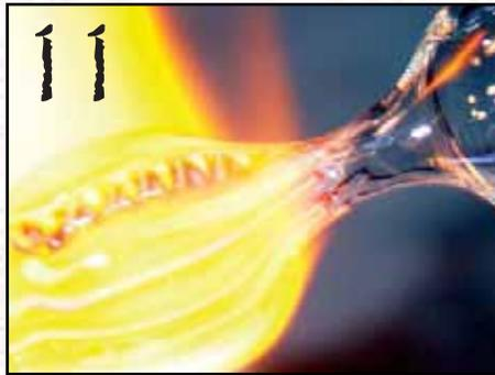
Focus heat on either side of the decoration. Allow the glass to constrict & draw down on each shoulder separately. Look for even wall thickness & diameter.
