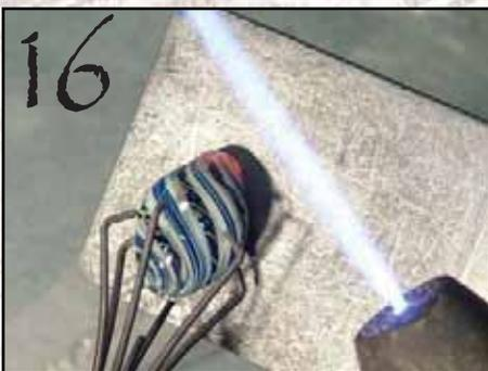
To adjust the size of the holes on either end of your bead, marver to make smaller, or use a tungsten pick or reverse tweezers to enlarge the hole.
