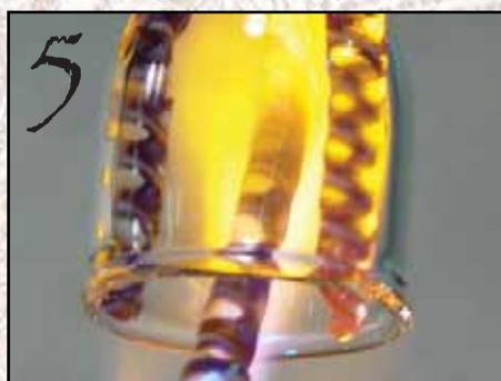
5 Using your prepared latticino, begin applying lines. Draw a total of 3 that are evenly spaced inside the point.
