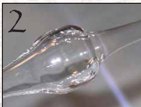
2 Using the same pinpoint flame, open each of the points at the thin shoulder area. Set one aside and seal the tapered end of the other point closed.
