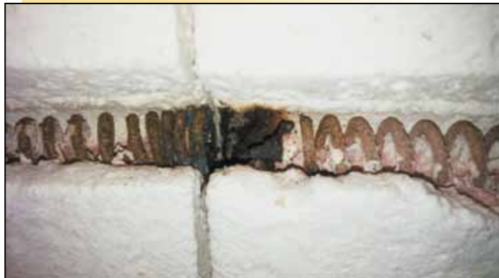
Nonstandard element pins will burn out an element. Photo courtesy of Jonathan Byler.
