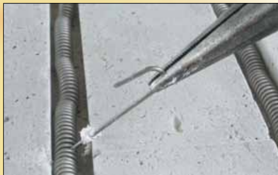
The earlier lid element grooves required pins. When replacing a pin, add a small amount of Pyrolite to the pin shaft. This helps to prevent the pin from falling out later.
