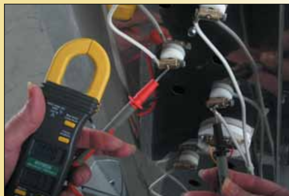
You can test the elements with an ohmmeter. This test is especially useful when considering buying a used kiln that you cannot plug in and fire before purchasing.
