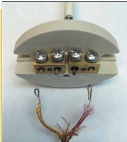
The thermocouple and the thermocouple wires going to the controller are color coded.
