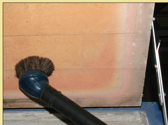
Vacuum the kiln after every six to ten firings or as often as needed to eliminate dust in the firing chamber.
