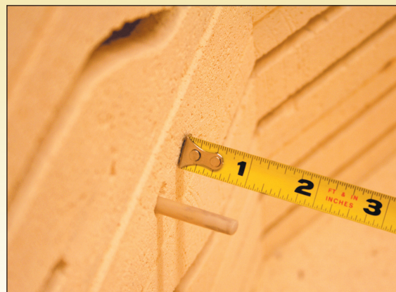
The thermocouple should extend into the firing chamber by four times its diameter.
