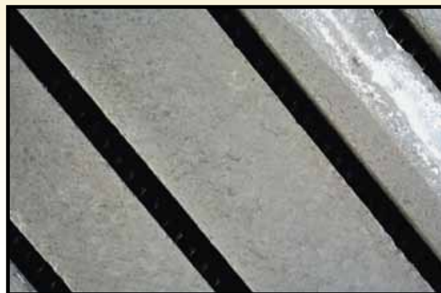
The coating on this lid has cracked because the coating is too thick.
