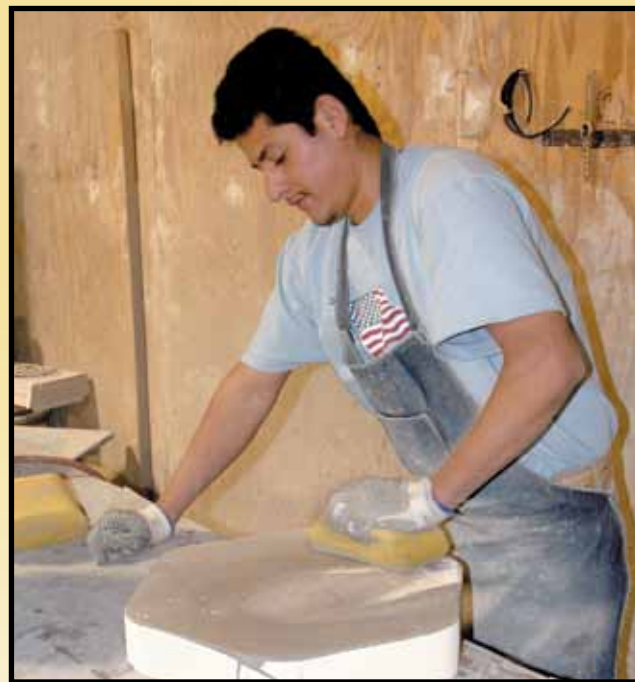
Use a large sponge to apply a thin coating to the firebrick lid.
